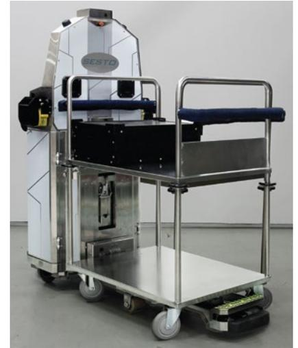
(L) Front view of Sesto AMR designed to autonomously transport trolleys
