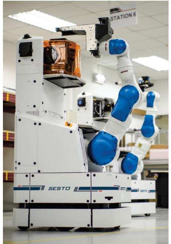
SESTO AMR equipped with 7-axis robot arm
